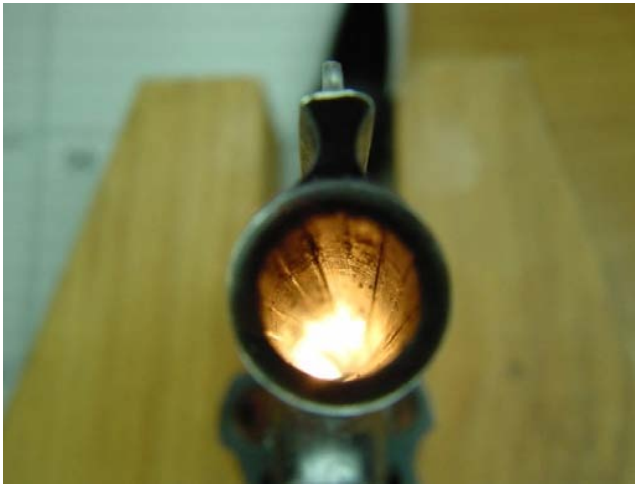
FIGURE 21.6 Spiral grooves are cut into the inner surface of a firearm barrel to impart spin to the bullet as it leaves the barrel, stabilizing its flight. The raised portions between the grooves are called lands. Courtesy: Richard Ernest, Alliance Forensics, Inc.
