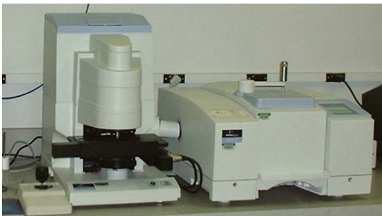
FIGURE 5.13 A Fourier Transform infrared spectrophotometer with attached microscope. Small objects such as single fibers can be mounted under the microscope, and high-quality infrared spectra can be obtained. Note that there is no ocular to see the sample through. Instead, there is a high-resolution camera mounted on top of the microscope. This is linked to the computer, which visualizes the image of the sample.
