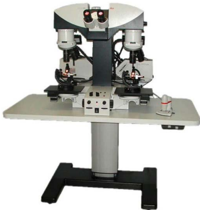
FIGURE 21.14 Much like the comparison microscope used for hairs and fibers work, the firearms comparison microscope optically joins two stereomicroscopes. This allows forensic scientists to view two objects simultaneously side by side. Courtesy: www.FirearmsID.com
