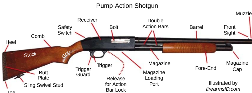
FIGURE 21.8 A shotgun is essentially a rifle that doesn't shoot bullets: Instead, it fires many small, round pellets or a single large slug. Therefore, shotgun barrels do not have rifling and have a limited effective firing range. Courtesy: www.FirearmsID.com, artwork by Erik Dahlberg
