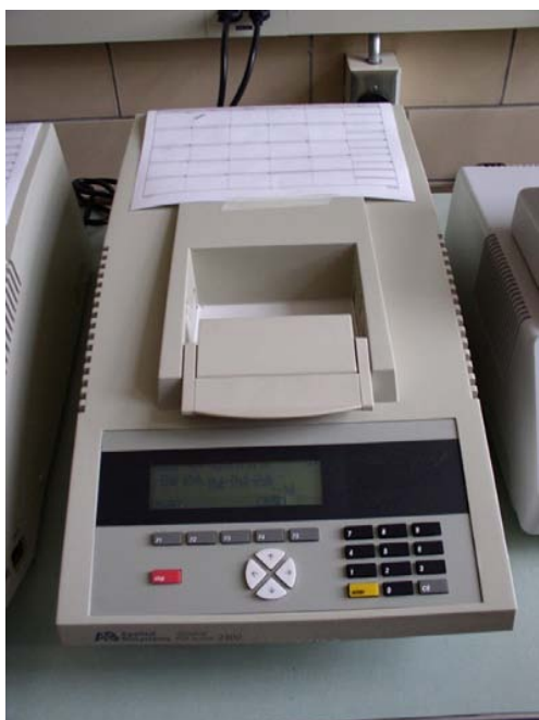
FIGURE 11.5 A thermal cycler. The main chamber holds metal blocks that contain vials with the reaction mixture. The built-in computer controls the temperature of the block and thus the vials. Each step of the PCR process requires a different temperature.
