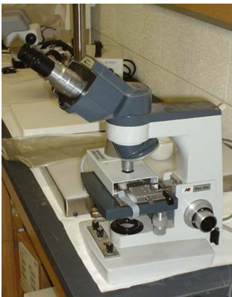
FIGURE 17.8 A hot stage and microscope. The hot stage is mounted on the microscope stage and is connected to a controller or computer that controls the rate of heating of the hot stage and keeps track of the refractive index of the liquid. The glass is immersed in a drop of liquid of known refractive index on a microscope slide, which then slides into the hot stage.
