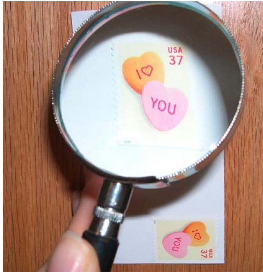
FIGURE 4.1 To see more detail in an object, here a postage stamp, the image must be magnified. This is accomplished with a simple hand lens, which enlarges the image 10 times, or 10 \times .
