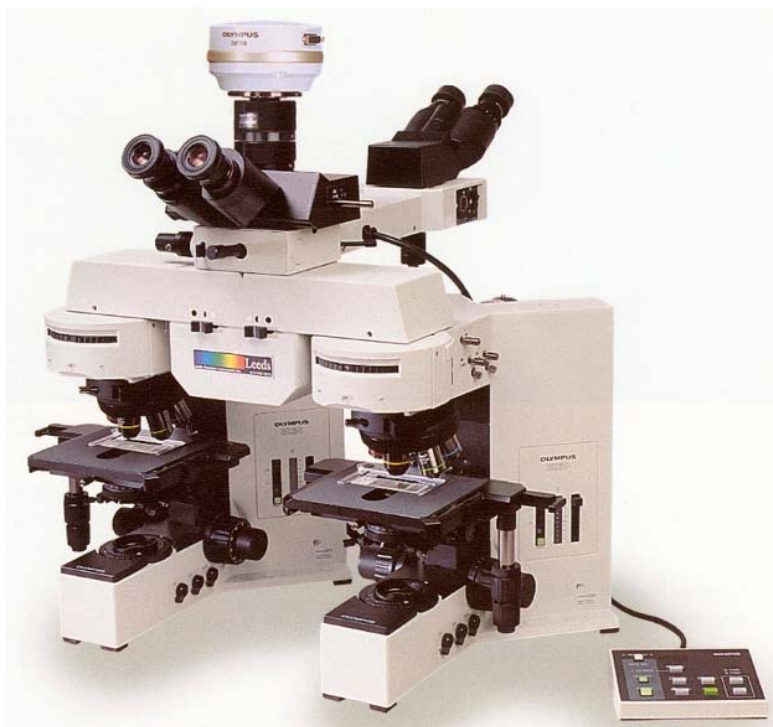
FIGURE 12.12 A comparison microscope is used for the examination. A comparison microscope is composed of two transmitted light microscopes joined by an optical bridge to produce a split image. The sample on the right appears in the right-hand field of view, and the sample on the left appears in the left-hand field of view. This side-by-side, point-by-point comparison is central to the effectiveness and accuracy of a forensic hair comparison. Hairs cannot be compared properly without one. (Courtesy: Olympus USA).
