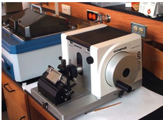
FIGURE 16.6 A microtome is a mini-vice that holds a sample in place while a heavy and very sharp glass or diamond-edged knife slices off sections a few tens of microns thick. Microtomes are useful for paint analysis by conserving sample consumption and preserving the samples for subsequent analyses. Courtesy: Olympus, Inc.
