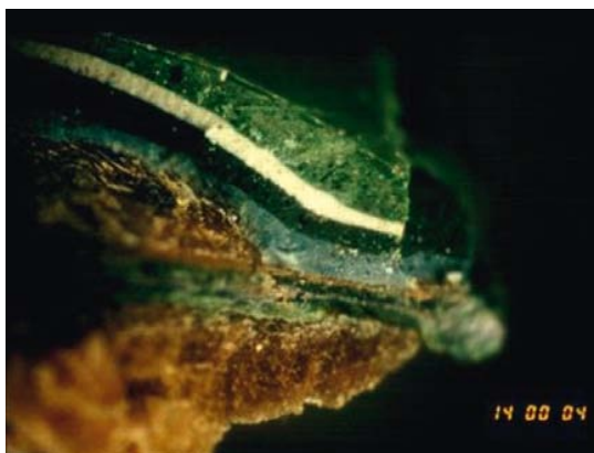
FIGURE 16.3 A green vehicle paint chip, showing the layer structure common to most automotive paints. Courtesy: Mark Sandercock, Royal Canadian Mounted Police.
