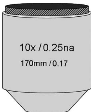
FIGURE 4.7 The objective lens, so called because it is closest to the object or specimen being viewed. The objective is the most important part of the microscope and comes in many types and magnifications. The information on the lens is very specific: “10×” is the magnification, “0.25na” is the numerical aperture, “170 mm” is the tube length (some objectives are now infinity-corrected and are labeled “∞”), and “0.17 mm” is the recommended thickness of cover slip to use.
