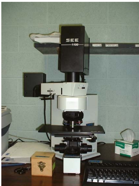
FIGURE 5.8 A UV/visible microspectrophotometer. The rectangular module on top is the UV/visible spectrophotometer. It sits upon a microscope, which focuses the light onto the sample. It is capable of absorption or reflectance spectroscopy.
