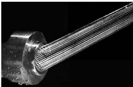
FIGURE 15.3 Synthetic fibers are formed by extruding a fiber-forming substance, called spinning dope, through a hole or holes in a shower-head-like device called a spinneret. This photograph appeared in the photographic essay, "The Reign of Chemistry," by W. Eugene Smith in Life Magazine , January 5, 1954.
