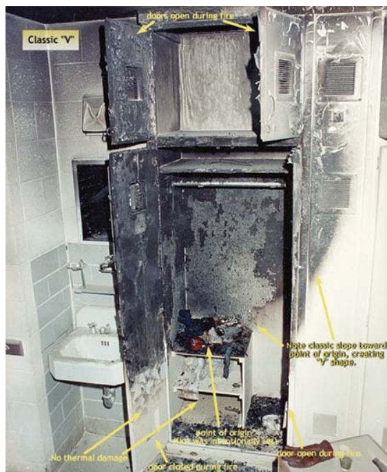
FIGURE 18.5 Point of origin of a fire showing the classic "V" burning pattern as fires burn up and out.
