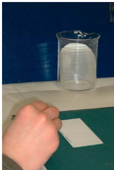
FIGURE 6.13 A thin layer chromatography apparatus. Note the piece of filter paper in the chamber (beaker). A small amount of mobile phase will be put in the chamber. The filter paper helps to saturate the space in the chamber. After the TLC plate is added, the chamber is tightly sealed.
