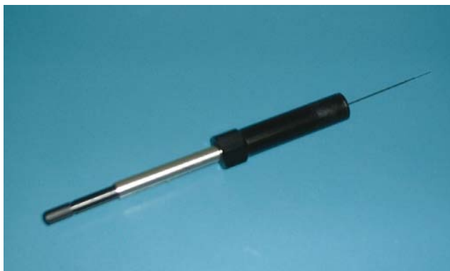
FIGURE 6.5 The solid phase microextraction apparatus. The fiber at the end of the wand can be coated with a particular polymer or other coating so that it will efficiently adsorb certain types of analytes. For example, there are SPME fibers that will adsorb molecules of flammable liquids mixed in with debris from a fire.
