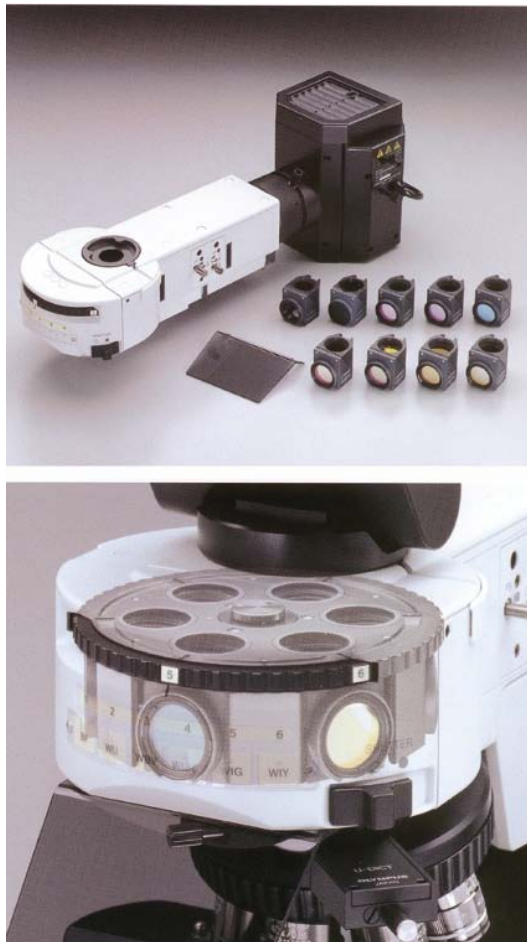
FIGURE 4.14 A fluorescence microscope uses various filters to exclude and excite specific wavelengths of light to induce fluorescence. Most microscope companies now package filters in sets, or cubes, to make choosing combinations easier. Courtesy Olympus USA.
