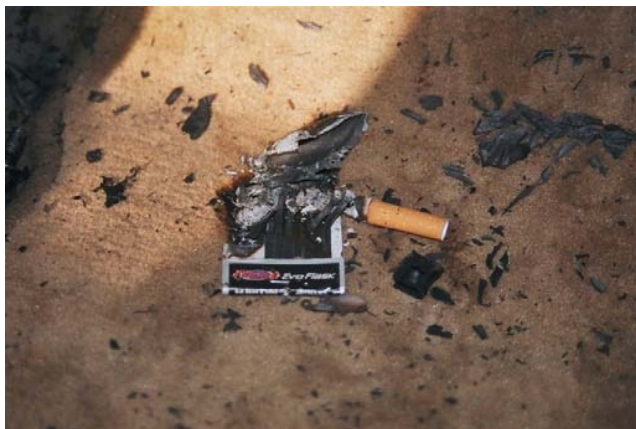
FIGURE 18.3 A timing device used to set a fire. An open pack of matches was put on the floor of a car near an accelerant. A cigarette was lit and put next to the matches. Eventually, the burning part of the cigarette lit the matches, which then set off the accelerant, causing the car fire. Courtesy: Lawrence D. Rossini, CFPS, Fire Investigator, Orange County Fire Investigation Unit
