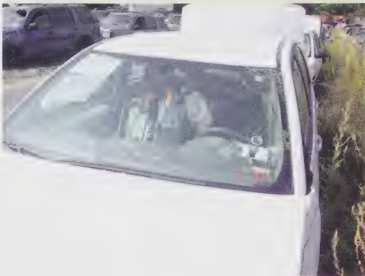
Figure 15-2a Broken laminated glass of a car windshield stays in its frame, protecting the car's passengers.
