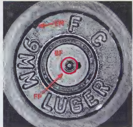
Figure 18-16 This cartridge shows three distinct impressions—the firing pin (FP), the breechblock face (BF), and the ejector mark (EM).
