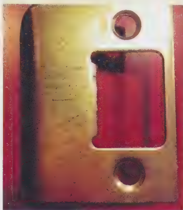
Figure 17-3 Abrasion: This door strike plate shows scratch marks made by a screwdriver.
