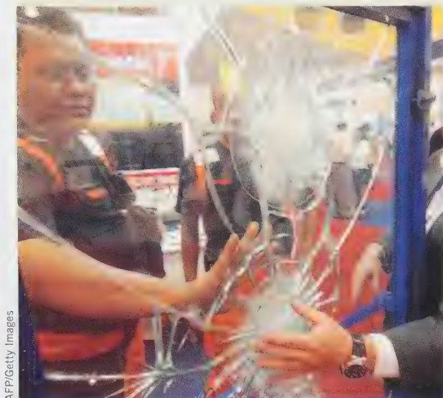
Figure 15-2c A bullet hole in bullet-resistant glass.
