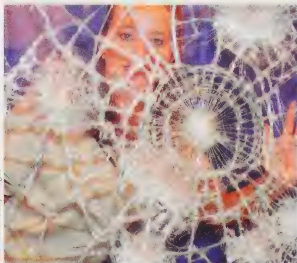
Figure 15-11 Note that the radial fracture lines originate in the center and extend outward. The concentric fractures are circles around the point of impact.
