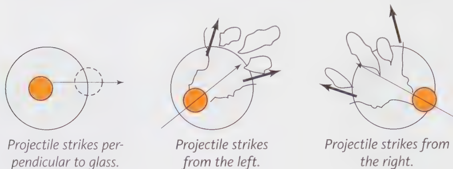
Figure 15-15 The glass pattern left by a projectile can help determine the position of the shooter. Note the entrance hole (tan) is smaller than the exit hole (dotted), and in this diagram, all the glass fragments appear on the exit side.
