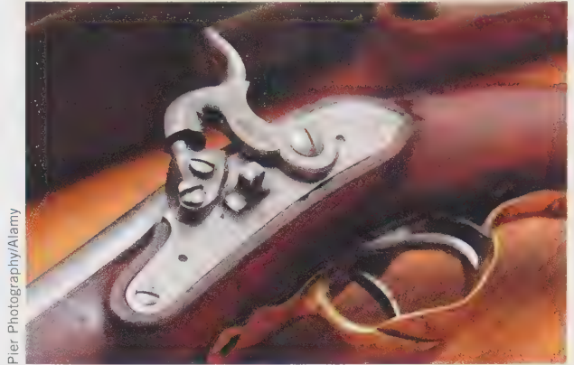
Figure 18-1 A percussion-cap firearm ignites the gunpowder using a primer that explodes when struck by a small hammer.
