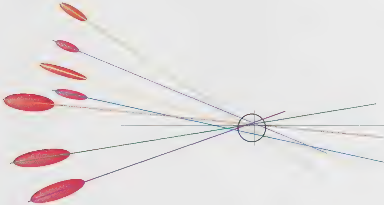
Figure 8-19 Area of convergence is estimated by drawing the smallest circle around the area where all lines through long axes of blood-spatter drops intersect.
