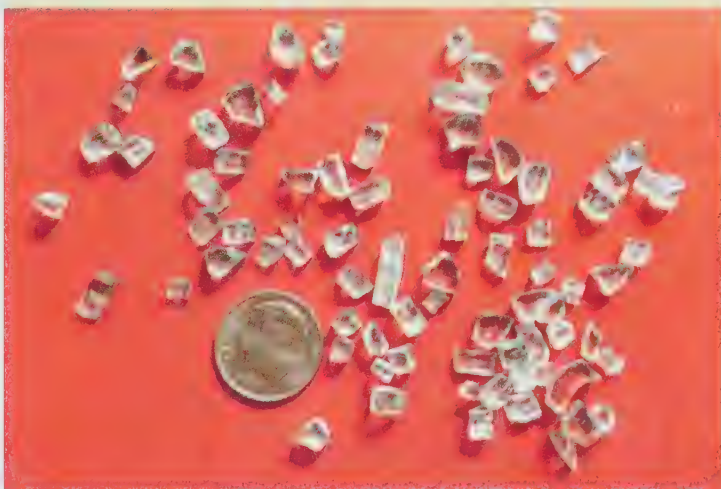
Figure 15-2b Broken tempered glass of a car's side window shatters into very small granules, or "pebbles." (A dime is shown for scale.)
