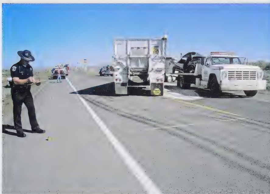
Figure 16-14 In a multiple-car collision, skid marks can help to determine the path and speed of each vehicle.
