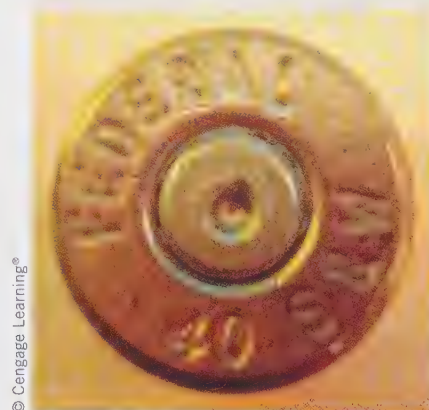
Centerfire impression on a .40-caliber cartridge.
