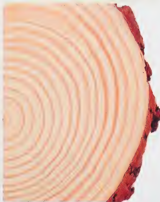
Figure 5-2 Annual rings: Springwood is a lighter-colored wood whose rings alternate with the darker rings of summerwood.
