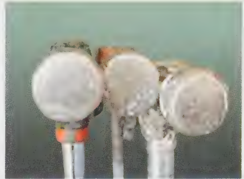
Figure 17-6 Unique markings such as nicks and ridge marks can be seen on the striking surface of these hammers.
