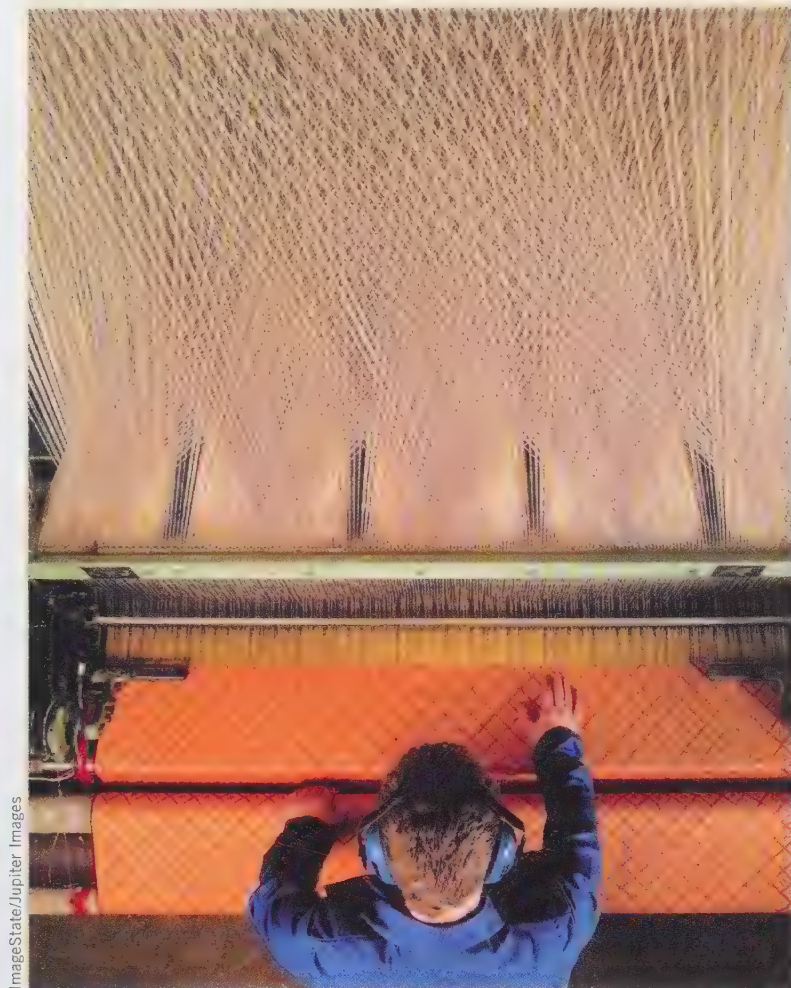
Figure 4-12 An industrial loom used to weave textiles.
