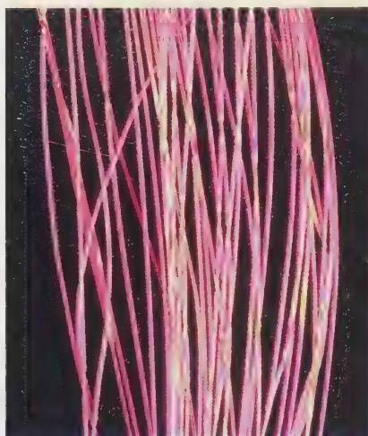
Figure 4-10 A polarized light micrograph of nylon fibers.
