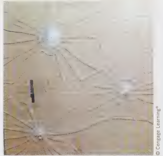
Figure 15-14 Three bullet holes and the fracture patterns they produced in glass.
