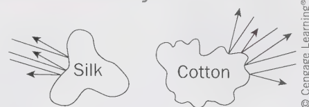
Figure 4-6 Cross-section of cotton and silk fibers.
