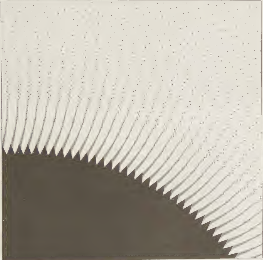
Figure 6.5 Even-sized droplets from the teeth of an ultra-low-volume pesticide sprayer
